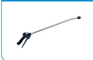
WHEEL CLEANING STAINLESS-STEEL LANCE. 600 mm + GUN F1/2". SIZE 03 FLAT 110° PLASTIC NOZZLE
