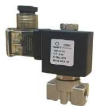
STAINLESS-STEEL SOLENOID VALVE. EPDM. 1/4"NC. 220V 0-16 BAR
