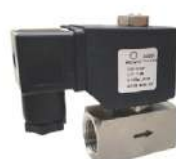
HIGH PRESSURE STAINLESS-STEEL SOLENOID VALVE. 0 - 120 BAR. PTFE (TEFLON). 1/2"NC. 24V AC.
