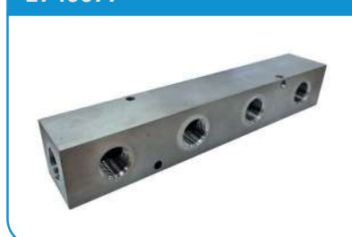
STAINLESS-STEEL MANIFOLD BLOCK. 4XF1/2" OUT + 2XF1/2" IN
